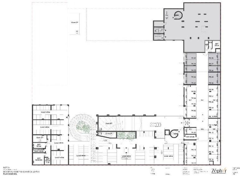
Layout of the entire underground area at Zephyr, including a few car parking spaces, 250 bicycle parking spaces and the mobility hub (top right)
